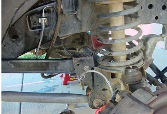
The **driver side** may or may not have dual inlets leading into the top of the hose, depending on whether the vehicle is 2 or 4 wheel ABS. The factory bracket may be in the way and may require the steel line to be slightly redirected. The driver side line feeds the passenger side caliper as well. Do not remove the frame mounted distribution block. Start by removing the passenger side hard line mount and attaching the new bracket
