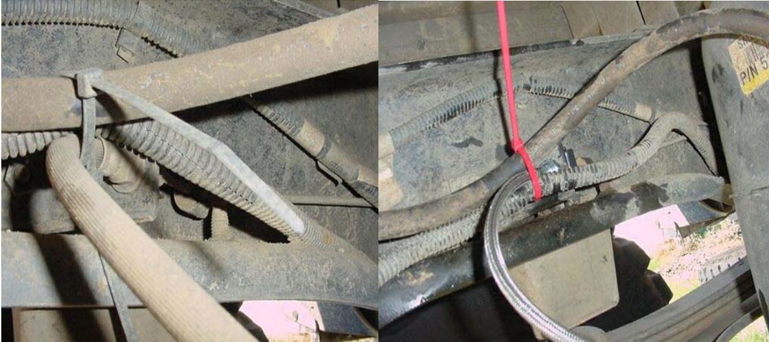
The frame end of the factory line is attached with a U-clip on the top of the fitting, loosen and remove the compression fitting from the block end of the line, pull the clip from the hard line to loosen and remove the hose. Connect the new hose end. Check for Proper Clearance and leaks! See ***Bleeding Instructions*** for tips and information on completely bleeding the system.
