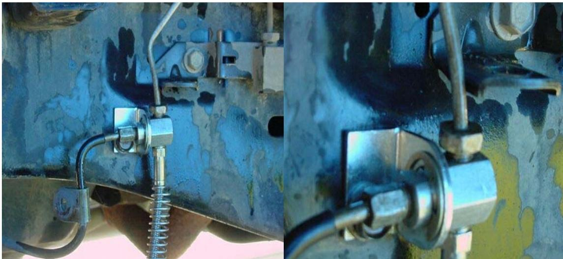
Attach the caliper end just like the passenger side, making sure you have properly routed the line. Swap the axle brackets. Use plenty of brake cleaner to
