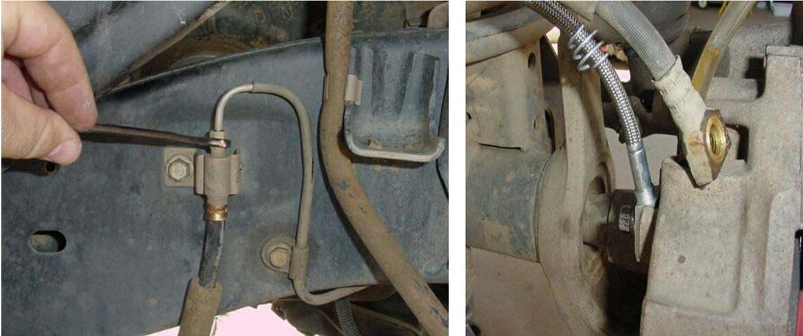
Unbolt the banjo bolt (7/16") attaching the rubber line to the caliper. Be sure to remove the washer from the caliper as well (there are two washers, one on each side of the line fitting. These washers should not be reused, and new ones are included. Once the fitting is loosened, and fluid in the line will continue to drain.
