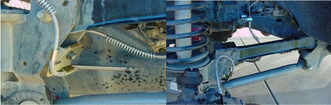
**Rear Hose-** clean the area around the rear distribution block and vent line to avoid getting debris into the gear oil. Start by removing the axle tube vent line. It is attached to a barbed fitting that passes through the rear brake line distribution block, holding it to the axle tube.
