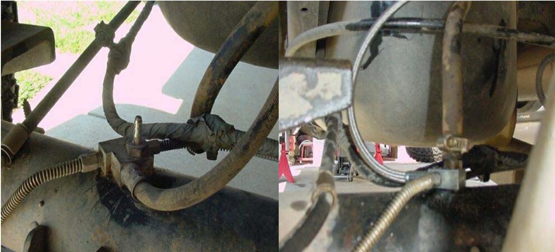
Remove the clamp, and then unscrew the barbed fitting from the block. Attach the hard lines to the new line. It is smaller than the factory hose, so the lines may need to be bent or adjusted to reach. Using the original vent fitting, attach the new line to the axle tube. Position the new line towards the front or rear of the truck, (depending on clearance). So that when the axle drops and pulls the line, the angle of the line to the block/frame mount is minimized.
