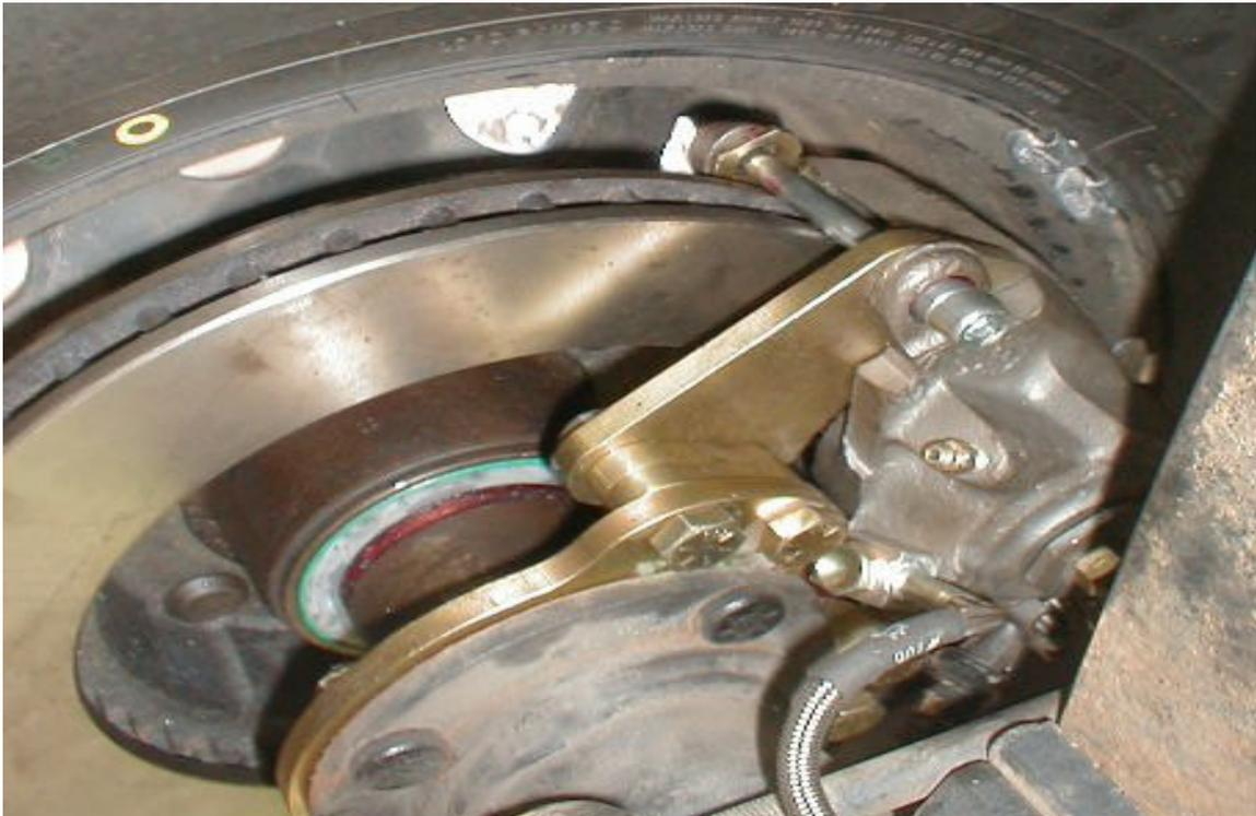
10. **Use P-Brake Cable Stop Nut** to take the slack out of cable between the end of the Cable Housing and the Caliper Actuator Arm. Cut end of cable off as required, (with grinder cut off wheel for a clean cut). Install Cable Stop Nut. \*May need to Space Spring Bracket out away from the caliper body with a couple of washers, to clear the P-Brake Cable and Bolt Heads.\* Custom made shorter cables are available from EGR Performance Brakes as well.
