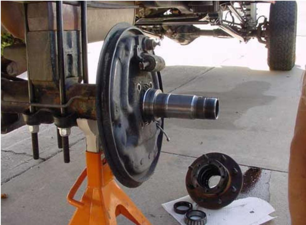
2. CHECK Rear Axle GVW on door tag.6000-6199# has 29/32" Stud Head. 6200# axle has 1-1/32" Stud Head & Bigger Knurl Section. Requires Turning Stud Head Down on Belt Sander or Grinder and Opening up Stud Holes in Rotor with 11/16" Drill Bit so knurl will drop through stud hole in rotor, TO PREVENT HOLE CRACKING.
